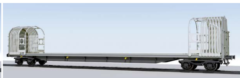
Railway SB · Example: Rils version for long goods, opened (on both sides)
