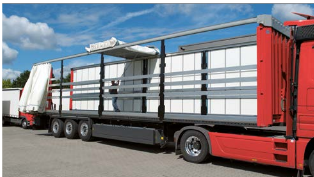
Opening of the roof and the side curtain using the CS-Hybrid as an example
