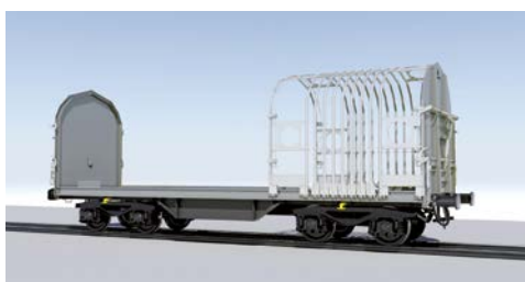
Railway SB · 示例: Shimmns 已打开的车顶
